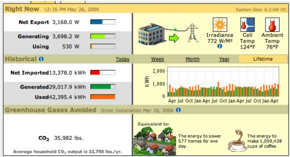
29,000 kWh generated & measured in May 2009 (top left), since a 2<sup>nd</sup> monitoring system was installed. For that sample May 2009 sunny On-peak moment, Irradiance is a sunny 772 W/M<sup>2</sup>, our PV is making 3,698 Watts, demand that moment is 530 Watts and 3,167 Watts is being exported. These exported Watts are valuable compared to high costs of gasoline! Put in an EV leveraging at Off peak rates, it accelerates time to PV payback.
