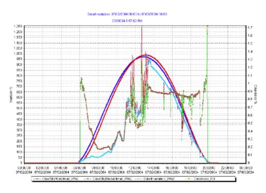
**Solar Irradiance (in green) that Same Day:** Corroborating clouding impacts 11 am - to 1 pm, sunshine drops well under theoretical maximum 1,000 watts/m<sup>2</sup> in same period. For more on Monocrystalline PV1 see our <u>rooftop performance graph series</u>.
