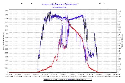
Sample Array Efficiency & Power over a Day, below: On a sample day roof mono PV 1 @ 14% module Efficiency was seen to outperform and do well 8 am — to 5 pm. While overall Efficiency (in blue) maintains a desirably flattened, broad parabola, Power output (in red) was more negatively influenced by the passing cloud cover from roughly 11 am — to 1 pm. Cloudy weather can have very sizably impact on PV:
